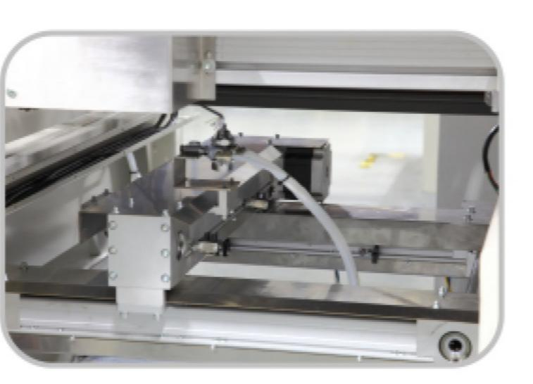
The spray system adopts the XYplatform + servo motor drive, which can be selectively spraying, and effectively save the flux.
