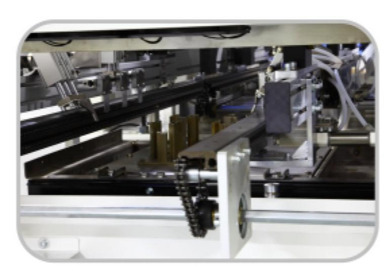
The position of the PCB allows a high accuracy and reliability, which is controlled by the clamping device from the aircylinder of X,Y,Z direction.
